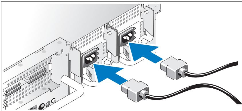
Connect the monitor (optional) and system power, and connect the system's power cable(s) to the system. If your system has an expansion card with a video output connector, *do not* connect the monitor to system's integrated video connector. Instead, connect the monitor cable to the connector on the expansion card.
