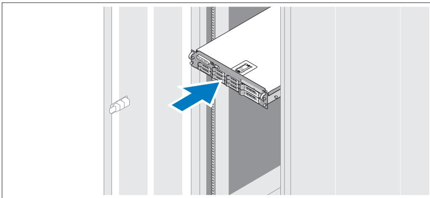
Once you have read the "Safety Instructions" located in the rack installation documentation for your system, install the rails and the system in the rack.
